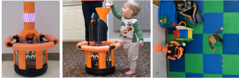
Fig. 1: Left: GoBot Bubbles, our custom robot with bubble, light, and sound stimulus hardware. Center: GoBot Throw, with ball-launching hardware. Right: Partial view of overhead play space with robot, participant, and toys.
